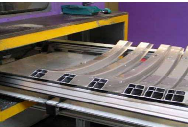
Fully automatized aluminium crash management production line
